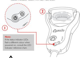
LEDs will flash fast green, ready to enter clearing mode. If clearing is not required, wait for the status indicator LEDs to revert to a slow green flash (Idle). Raise Solo 365 again to begin clearing, indicated by fast white flashing status indicator LEDs.
