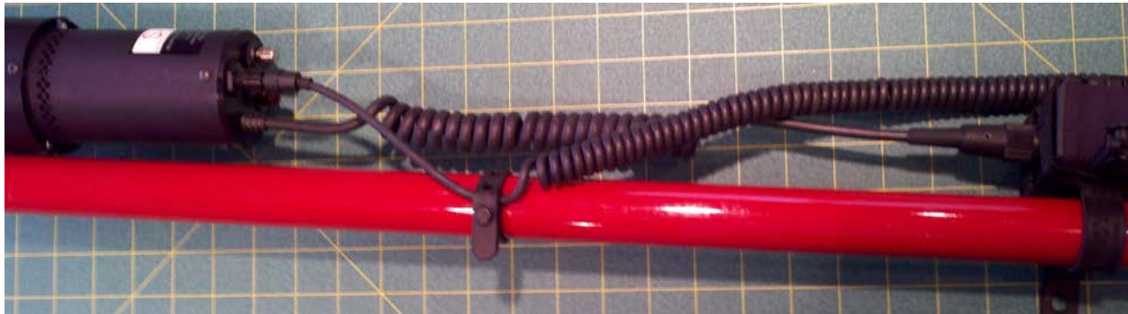
Picture 1: Fasten the axial cable lead to the pole using the rubber strap provided. Note that the actual cable has longer axial lead than pictured to provide for swivel movement of test head
